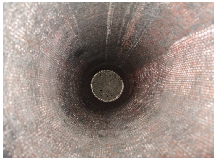
The inner surface of FuranFlex lining after 1000 °C heat test upper 1 m section
