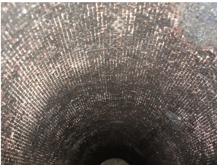
The inner surface of FuranFlex lining after 1000 °C heat test upper 1 m section
