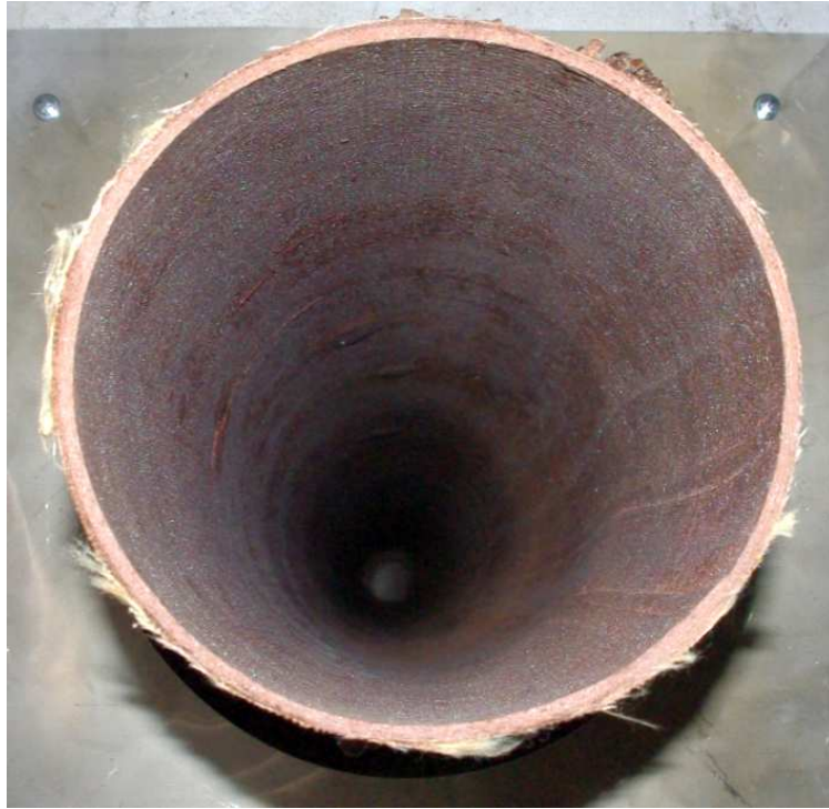
The inner surface of FuranFlex lining before the test (end section)
